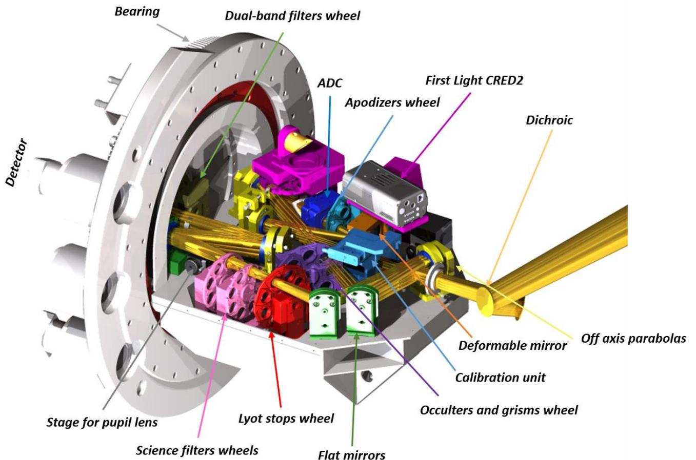
Figure 3: the opto-mechanical concept of the SHARK-NIR optical bench.
