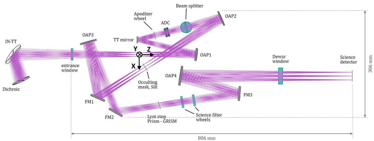
Figure 2: Optical layout of SHARK-NIR (top view of the optical bench). The light beam enters the instrument on the left side of the figure.
