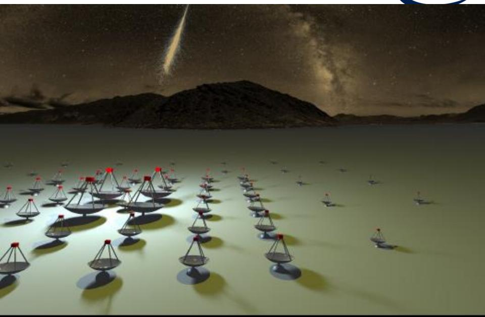
Low-energy section: 4 x 23 m tel. (LST) - Parabolic reflector - FOV: 4-5 degrees energy threshold of some 10 GeV
