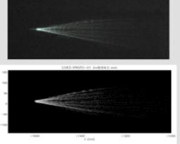
Comparison between optical measurement and ray-tracing from surface measurement
