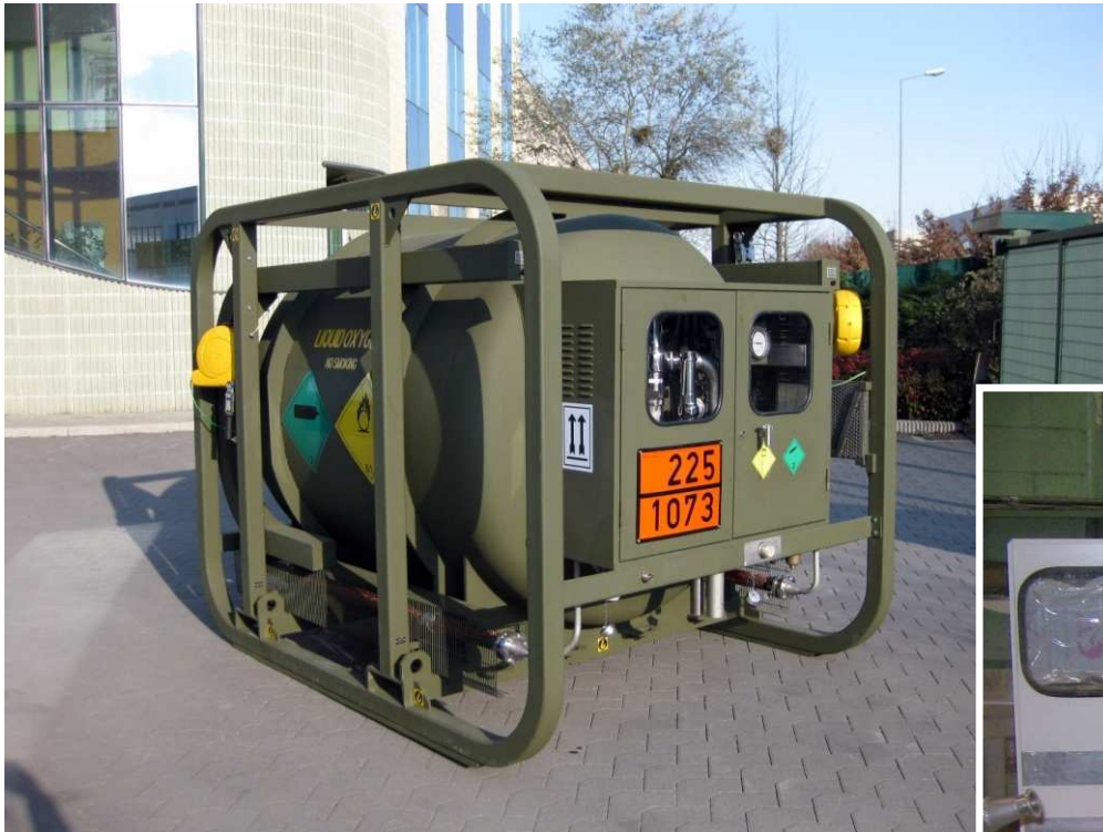
500 gls LOx reservoir for Air transport – AMI (2008)
