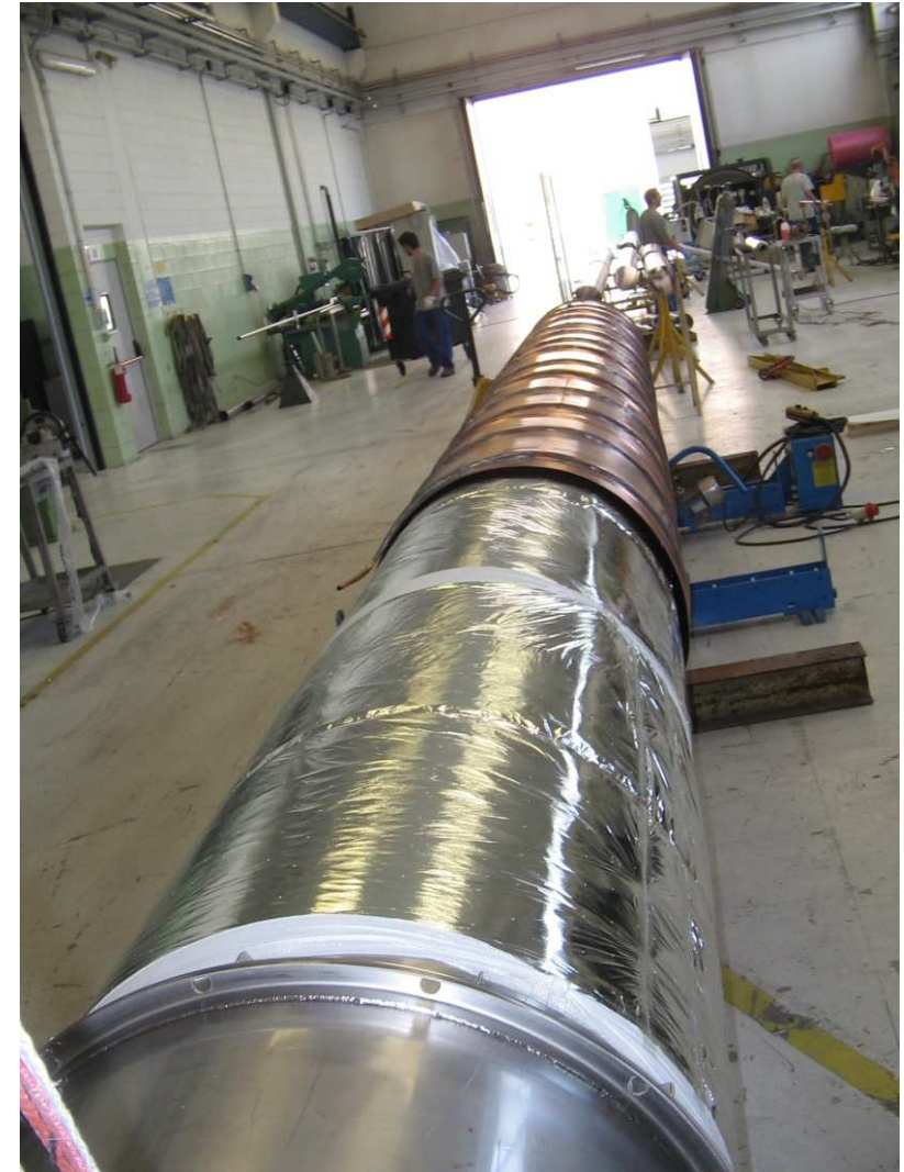
Liquid Helium cryostat for superconductivity test – INFN (2010)
