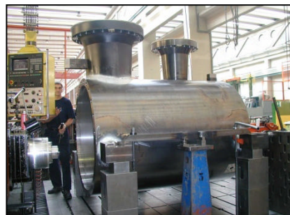
Compressor casings Barrel type (forged, welded and machined)
