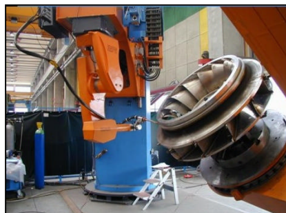
Francis, Pelton , Kaplan impellers (forged, welded and machined)
