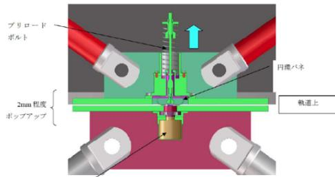
Truss separation mechanism
