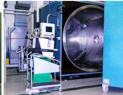
Large TV facility, 6 m 3 vol, 1 mbar, +100C / -35C for balloon instr.
