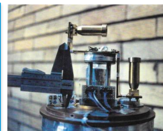
3 He sorption refrigerator for balloon flight cryostat
