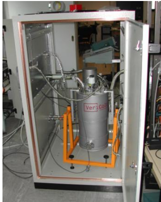
PT + ADR (< 50 mK, Vericold) for detectors test in shielded cage
