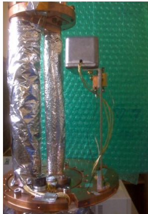
Pulse tube (~2.4 K) for cryo electronics test
