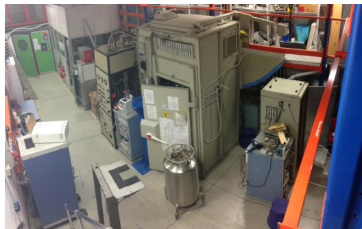
Test facilities (3 dilution fridgew)
