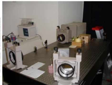
Figure 4.8: : The ZYGO GPI-XP interferometer. Layout (left) and photo (right) of the ZYGO interferometer.
