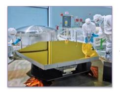
Each one of the 18 segment has 7 controllable degrees of freedom and the secondary mirror has an additional 6 degrees of freedom
