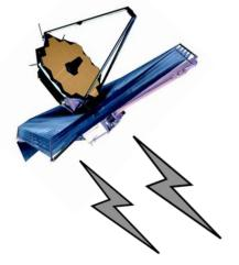
**Low rate S-band** up/downlink for commands, real time telemetry
