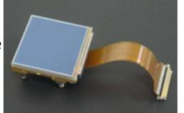
The METIS **UV detector** (UVD) will be a photon counting Intensified Active Pixel Sensor (IAPS) with a  $2k \times 2k$  format, 15  $\mu$ m pixel size, with the capability of working also in integration/analog mode under high flux though with a reduced spatial resolution (30  $\mu$ m pixel size, 1kx1k)
