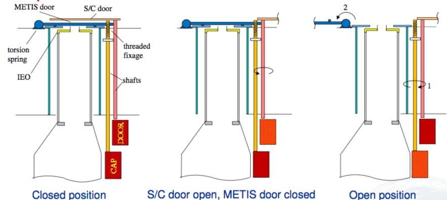
Impacts on the spacecraft: modification of the feedthrough top cover (addition of METIS door hinge); accommodation of an additional shaft of an additional motor; external door height above heat shield increased. Note: an internal motor + shaft could be used also for retaining/releasing the ejectable cap in place of the pin puller.
