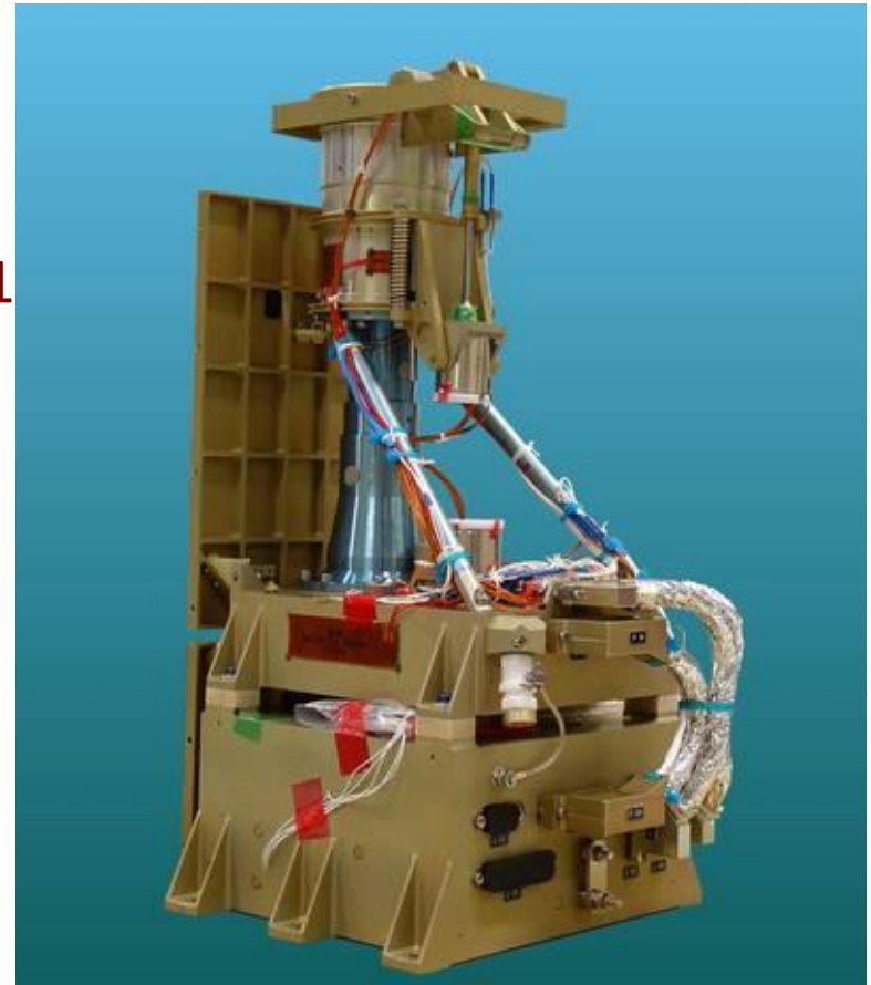
One of the FCs; 1k x 1k CCD with a huge range of integration times (1ms to 3.5 hours).
