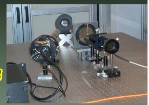
Development and test of a Liquid Crystals Tunable Polarimeter LCTP
