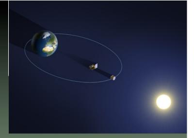
Moving the occulter further away preserving eclipse-like conditions for long periods is the performance offered by the Proba-3 ext. occ. coronagraph.
