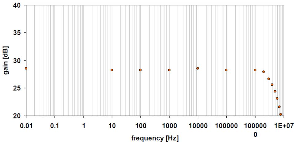
Frequency response from DC to 10 MHz at Troom and at low power ( $\sim 1\text{mW}$ ). The -3 dB point in this condition is around 4 MHz.  $G \sim 25\text{ V/V}$
