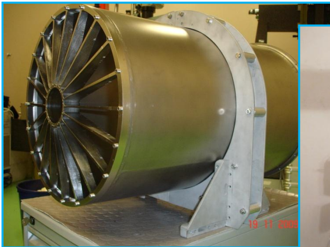
Mechanical structure: 2 spiders with 20 spokes
