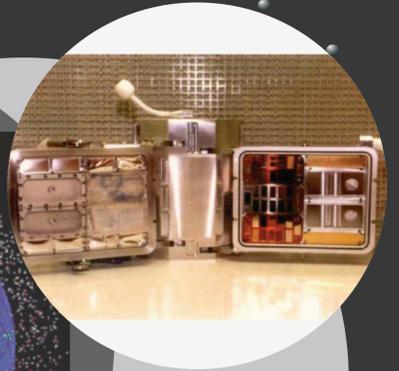
**AEROGEL** catching systems have been externally exposed on the Russian space station MIR, to catch grains of natural origin and/or fragments produced by space human activities (so-called debris)
